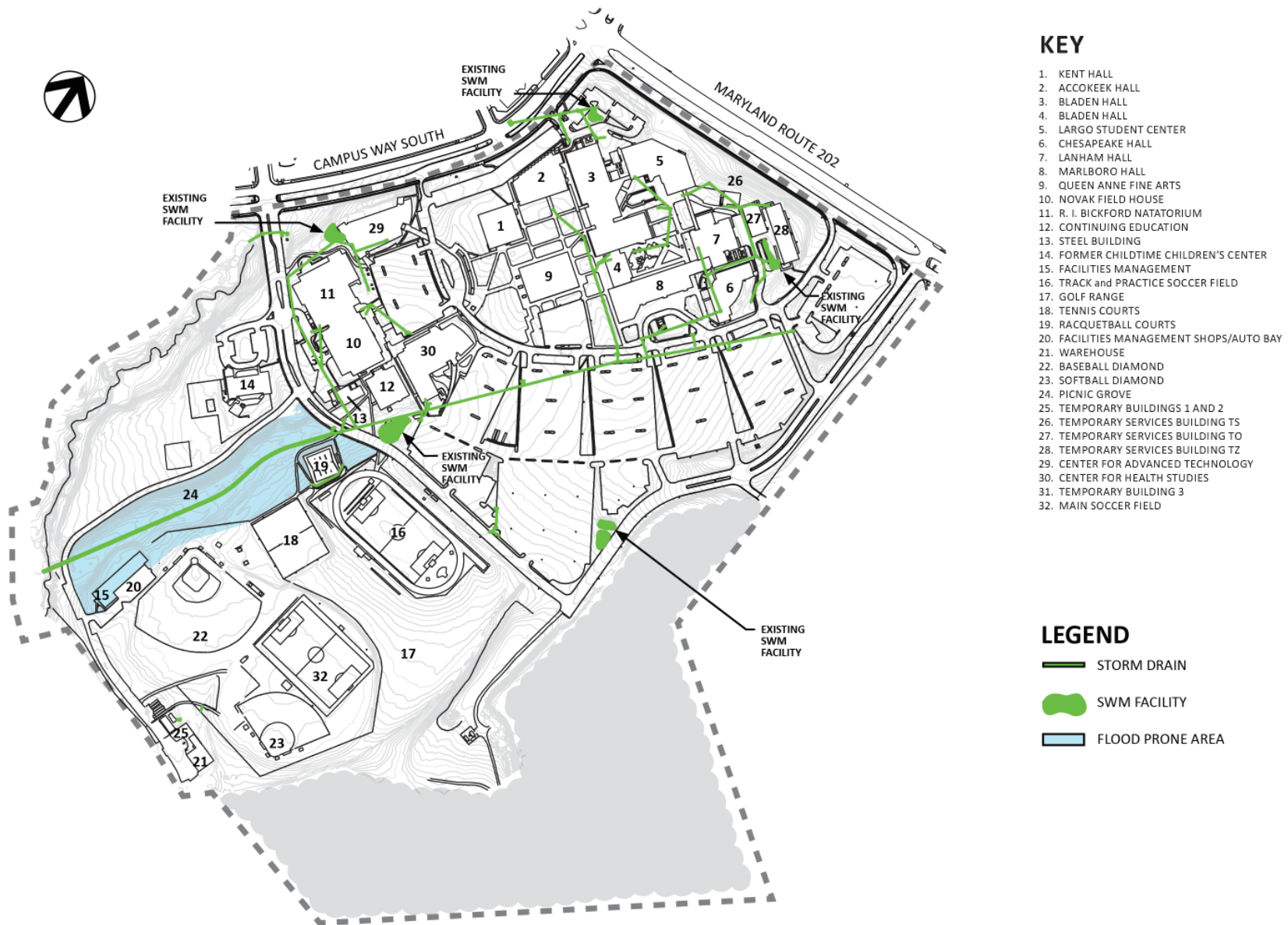
Figure 4.10 Largo Campus Existing Stormwater
