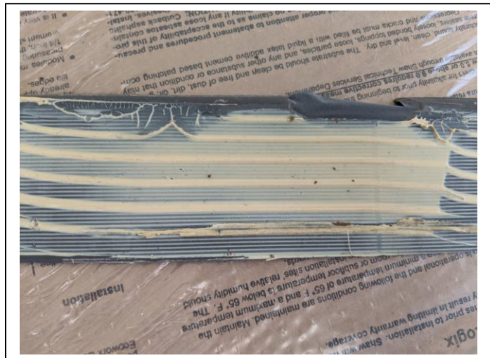
Photo #26 Material: Tan baseboard mastic Sample location: AMA S-1 No Asbestos Detected
