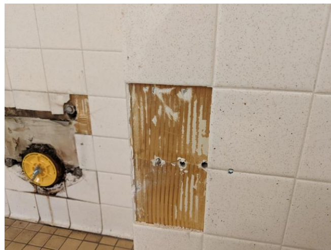
Photo #46 Material: Yellow ceramic tile mastic Sample location: AMA 2-13 No Asbestos Detected
