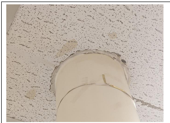
Photo #43 Material: White pillar caulk Sample location: AMA 1-58 No Asbestos Detected
