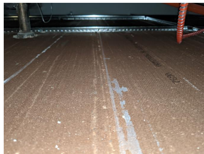
Photo #31 Material: 2'x4' Cratered/pinholed ceiling tile (brown backing) Sample location: AMA 2-48 No Asbestos Detected
