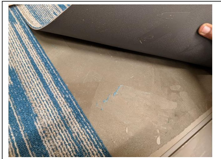
Photo #25 Material: Blue carpet mastic Sample location: AMA 1-27 No Asbestos Detected
