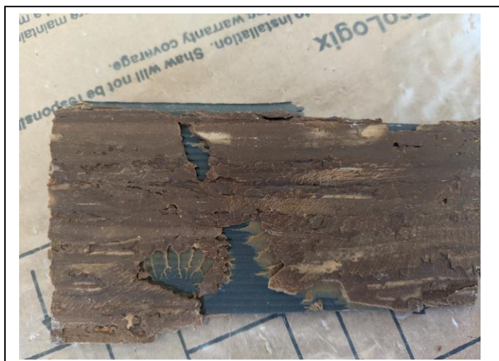
Photo #27 Material: Brown baseboard mastic Sample location: AMA S-1 No Asbestos Detected
