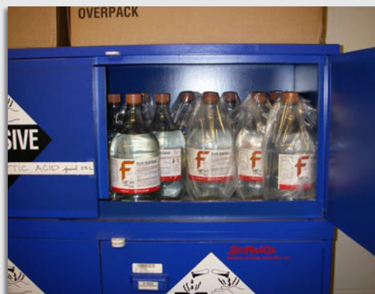
Store bases in a corrosives cabinet.
