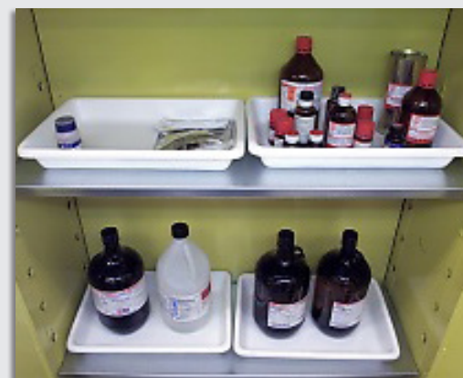
Store chemicals on spill trays to contain leaks or drips.
