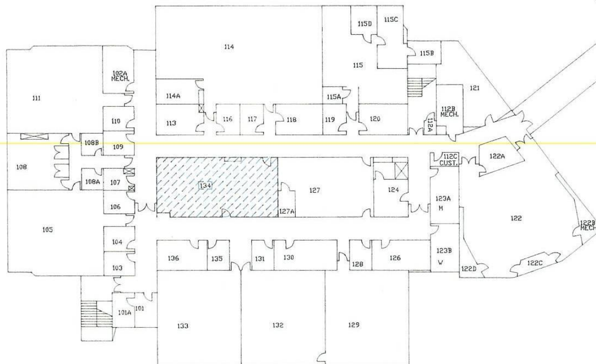
FIRST FLOOR AREAS POSITIVE FOR TRANSITE INSIDE FUME HOODS
