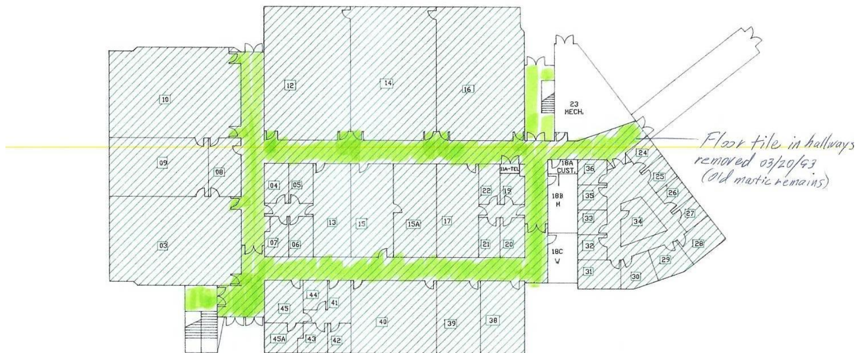
GROUND FLOOR AREAS POSITIVE FOR FLOOR TILE AND MASTIC (ASSUMED)
